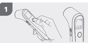
**EN** Press the power/test button and wait until display is activated
