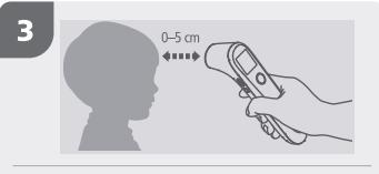
**EN** Aim at the forehead/object with a distance less than 5 cm and press test button
